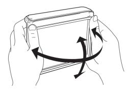
4. Turning the display downward. Make sure to return the display to centre position before drawing in. It cannot be draw in with its angles adjusted.
